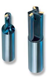
The large chip flutes in combination with embedded clamping elements guarantee an excellent chip evacuation. The clamping element has to be slightly released only in order to change the insert. However, the clamping element itself remains securely connected to the holder.
