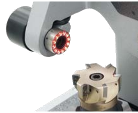
Cutting edge inspection
